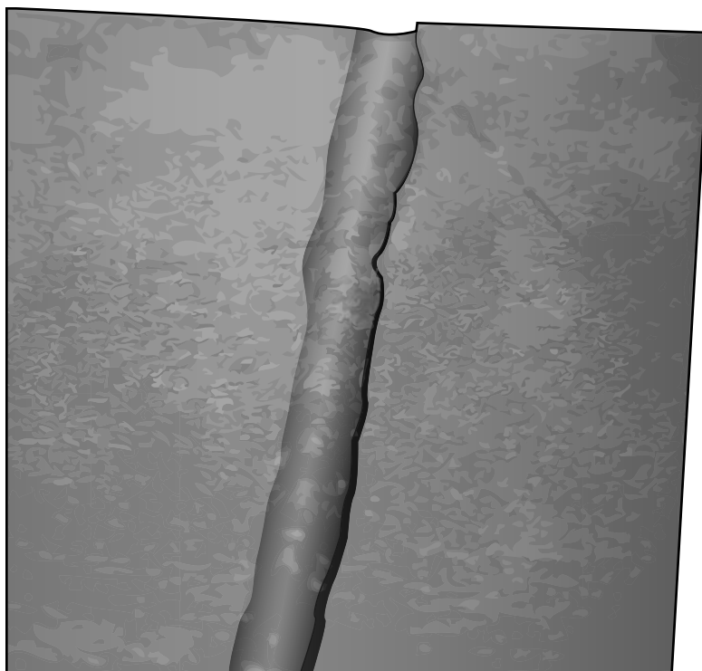
Figure 18-3: Example of a crack along a weld.
