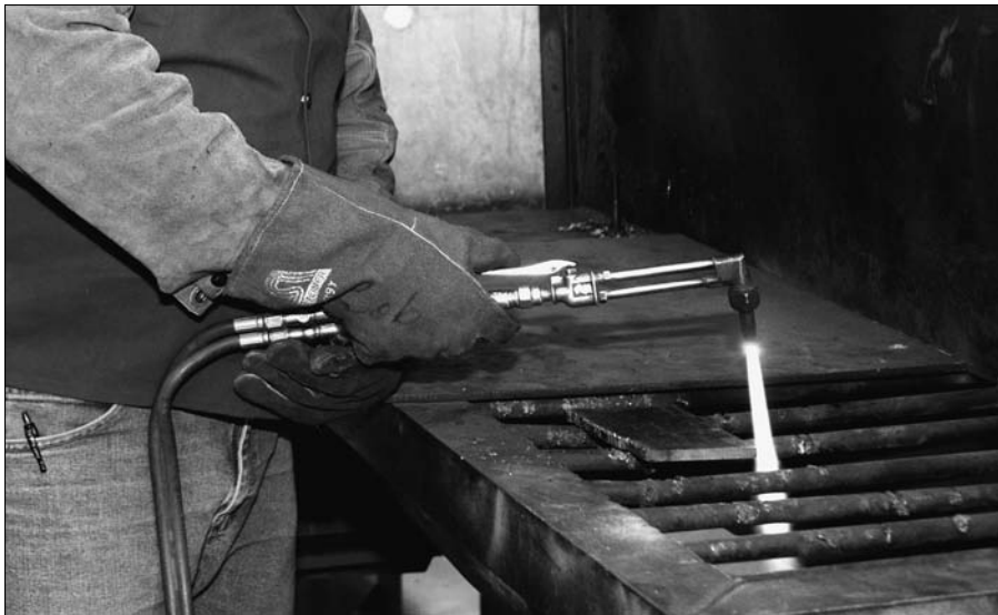
Figure 12-4: Operating an oxyfuel cutting torch.
