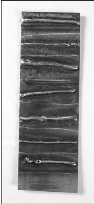
Figure 10-2: Examples of mig weld beads, from top to bottom: Good, too fast, too slow, voltage too low, voltage too high, WFS too low, WFS too high
