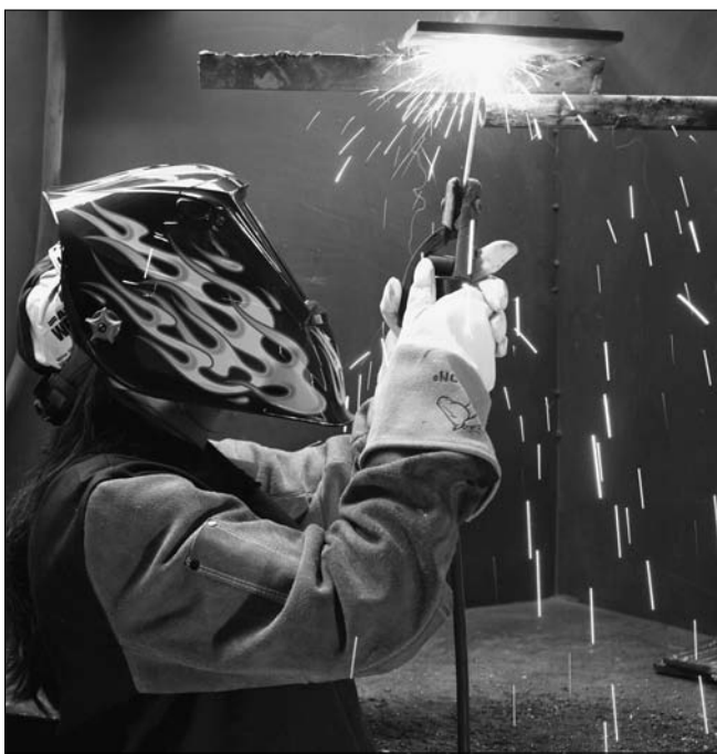
Figure 6-8: Practicing overhead stick welding.
