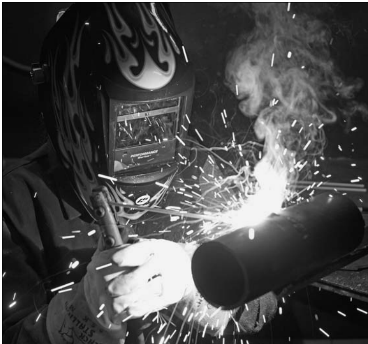
Figure 14-1: Steel pipe being stick welded.
