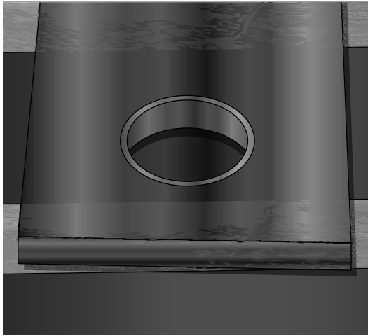
Figure 12-2: Perfect circle cut in aluminum.
