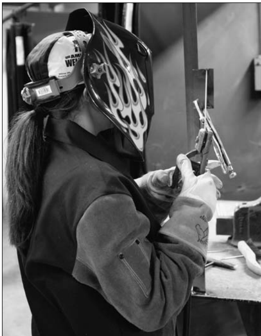
Figure 6-6: Practicing vertical- down stick welding.
