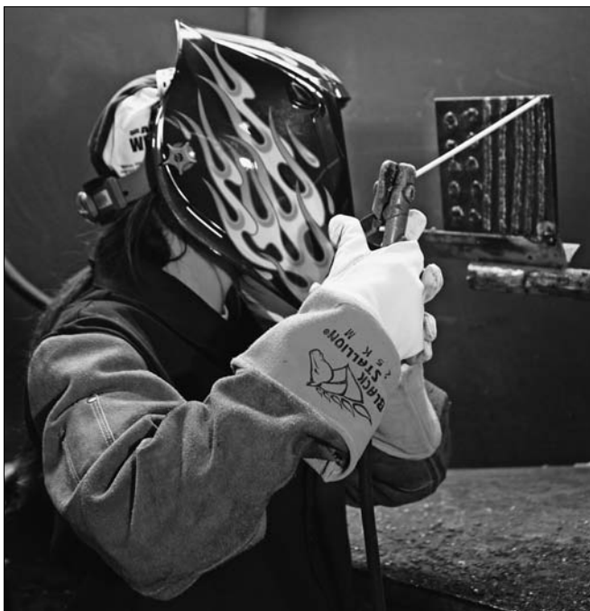
Figure 6-5: Practicing vertical-up welding.
